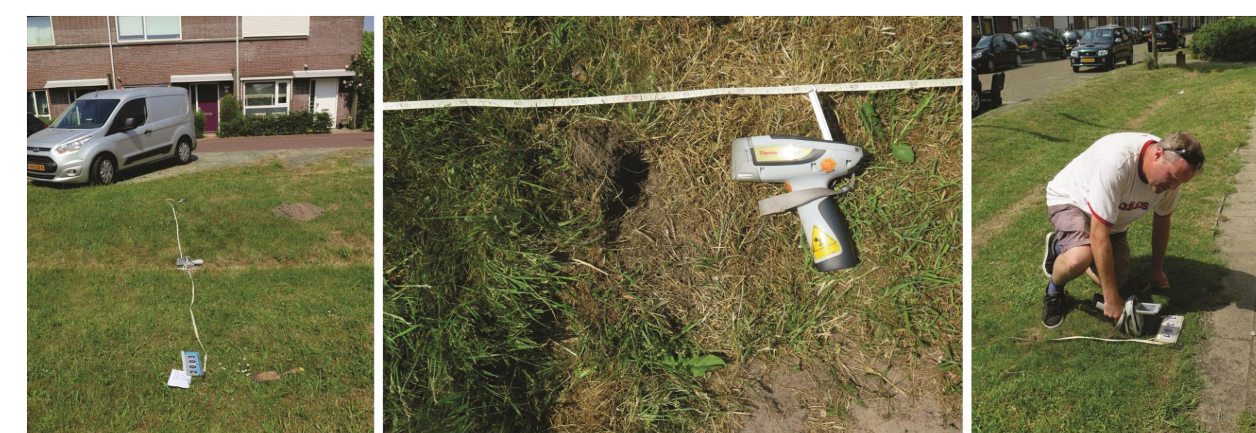
Figure: Demonstration of in situ XRF measurements at every 1 metre along the profile across the swale. The vegetation is removed to measure on the topsoil, 0-3 cm, for measuring results to be comparable with lab results from soil samples. The instrument is pointed on the topsoil and each measurement is read for 60 seconds.
